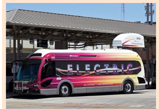
A Proterra electric bus operated by the San Joaquin Regional Transit District (RTD) recharging at a fast charging station. The RTD’s e-buses entered into service in 2013. Photo: San Joaquin RTD (2013).
